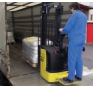
Increased under clearance (MWS14/20FA-1R)
