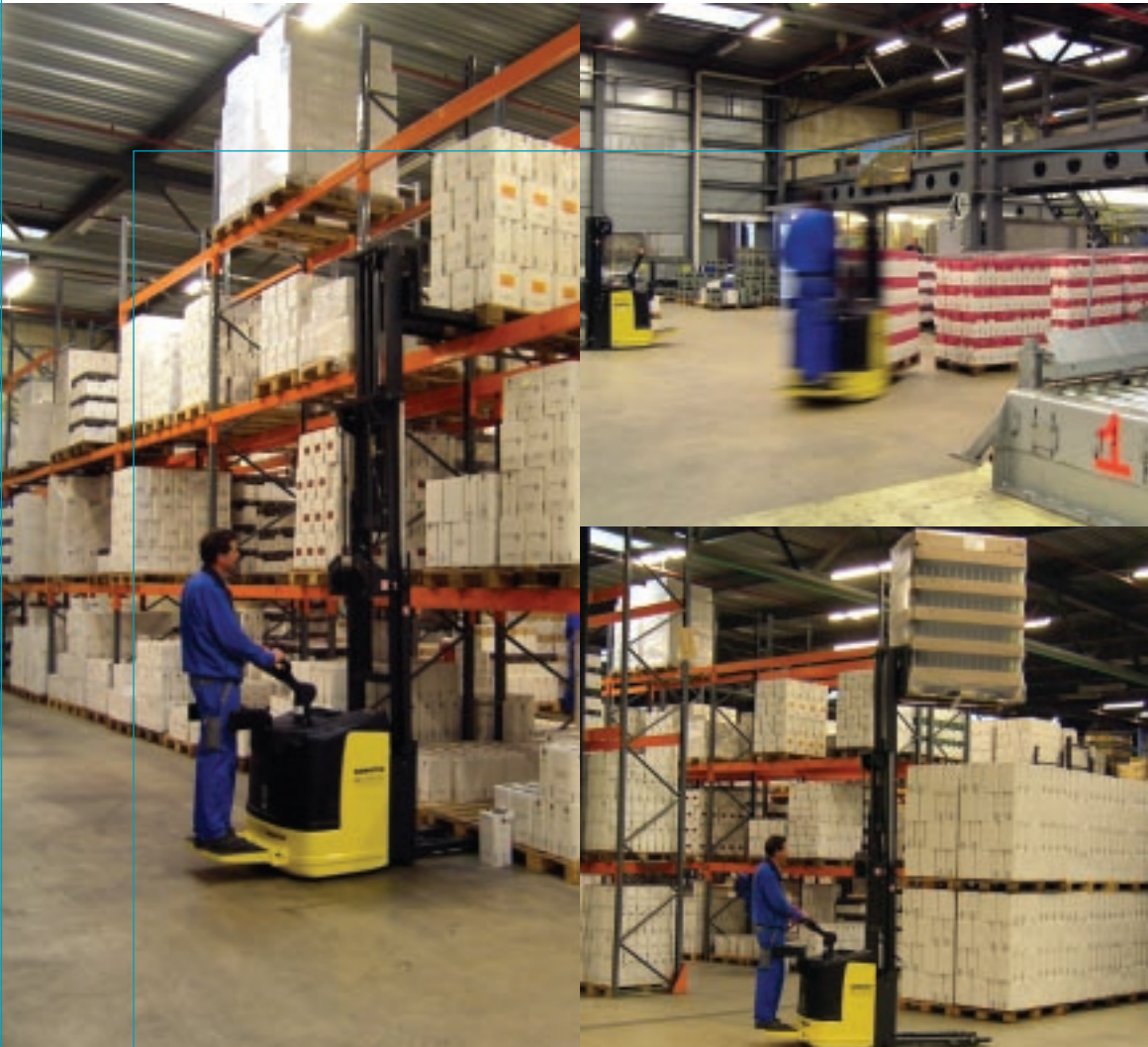
Pedestrian Stacker Truck with Folding Platform with/without initial lift
